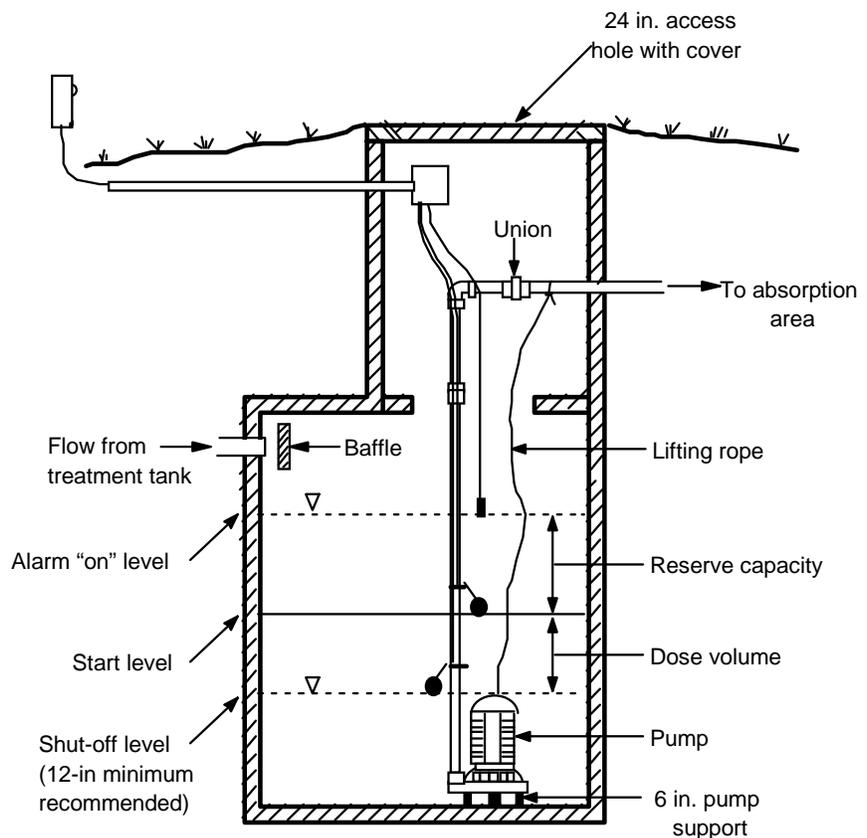
Figure 2. Pump tank for a sand mound.
